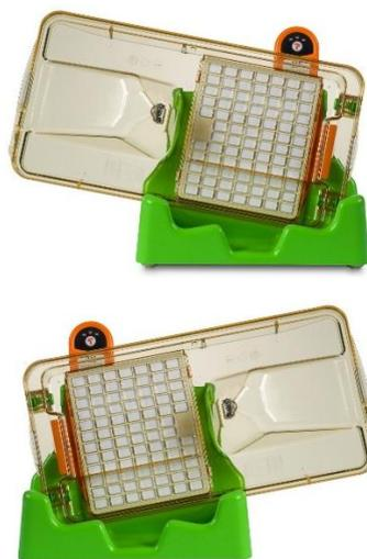
The RED LED stays fixed as soon as the RFID Reader reads the IVC Cage top RFID tag. A window with the cage information is displayed in the DVC® OPERATOR interface (only when the RFID Reader is already associated with the user).
