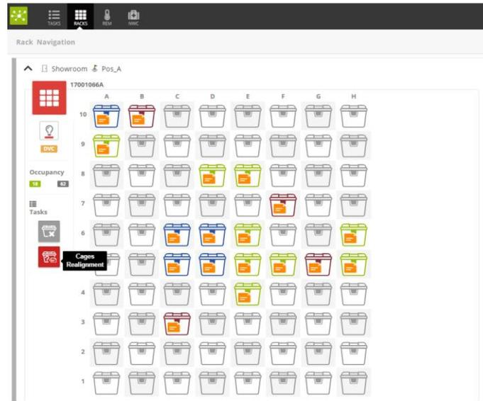
The DVC® Operator interface changes to a dedicated page where the user is requested to click on the empty cage to be updated. By doing so, the corresponding cage is highlighted in the DVC® Rack view, and two different search areas appear.
