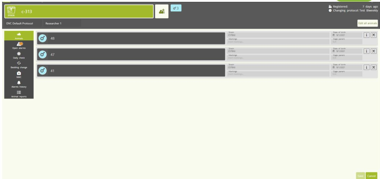
Suppose the user searches for multiple elements (such as cages belonging to a protocol or an Owner). In that case, the result can be a list of cages, always grouped at DVC® Rack level that can be illuminated altogether by clicking on the upper icon
