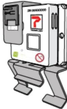
The first step is to attach the REM to the DVC® Master following the procedure described in the REM manual.
