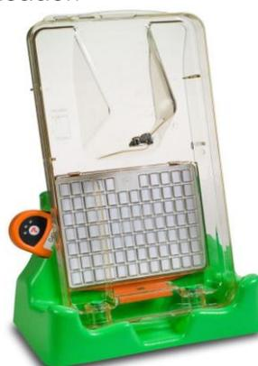
If the cage top is placed horizontally (lying on its side), the RFID Reader needs to be put in the top housings as shown.
